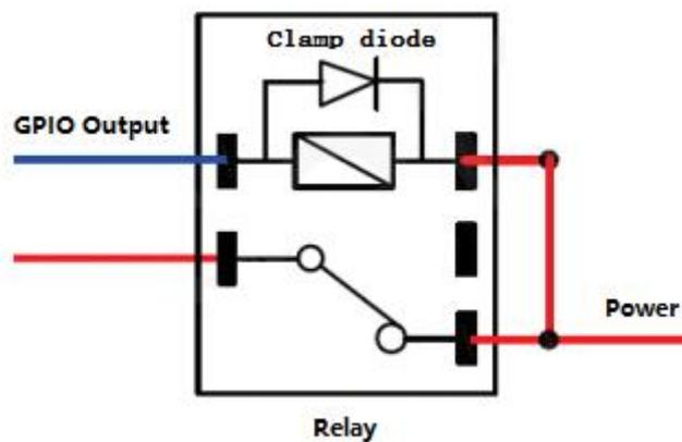
Figure 3.11 Typical Relay Connection
